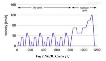
Acceleration, constant speed and braking time periods are displayed by fig.2, which describes the average run of city and highways. There should be less braking moments via the electric motors during cycle of the braking, in area where velocity of car is decreasing. The way for more energy generation is more braking moment's bye electric generators of the electric powertrain. [5, 6]
